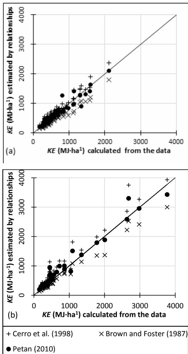
**Figure 4:** Example of results for three selected *KE-I* relationships plotted versus *KE* estimated using the disdrometer data from Ljubljana (a) and from Črni vrh (b).
