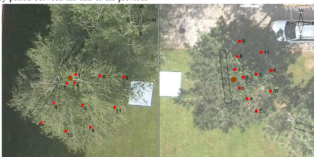
Figure 1: Location of the funnel-type throughfall gauges, marked with red points (left birch tree, right pine tree). Black lines indicates the position of through gauges.
