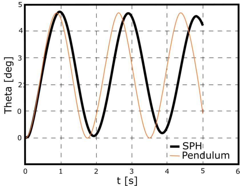
**Figure 4:** Manoeuvre 1: comparison of gravity centre oscillations between the SPH and dynamic pendulum; 20% filling height.
