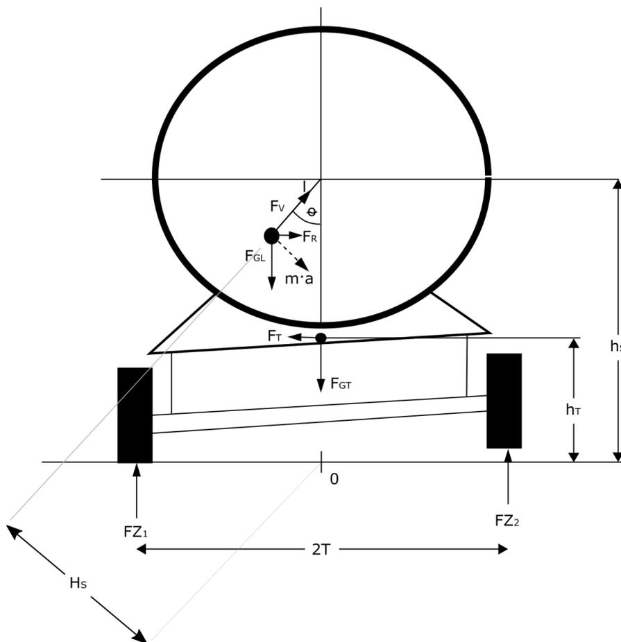
**Figure 2:** Overturning mechanism in the pendulum method.
