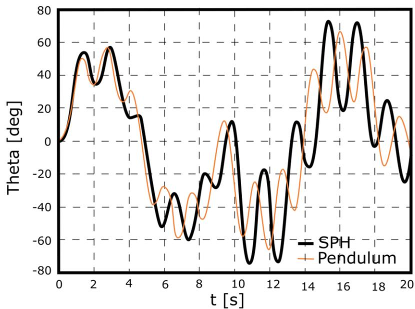
**Figure 7:** Manoeuvre 2: comparison of gravity centre oscillations between the SPH and dynamic pendulum; 20% filling height.
