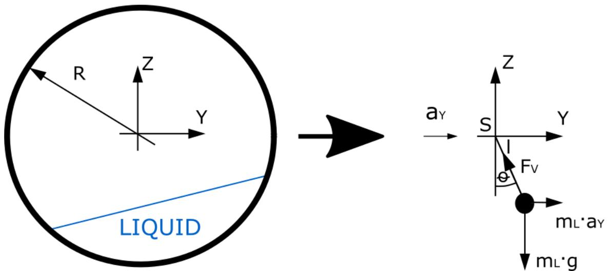
**Figure 1:** Pendulum model.
