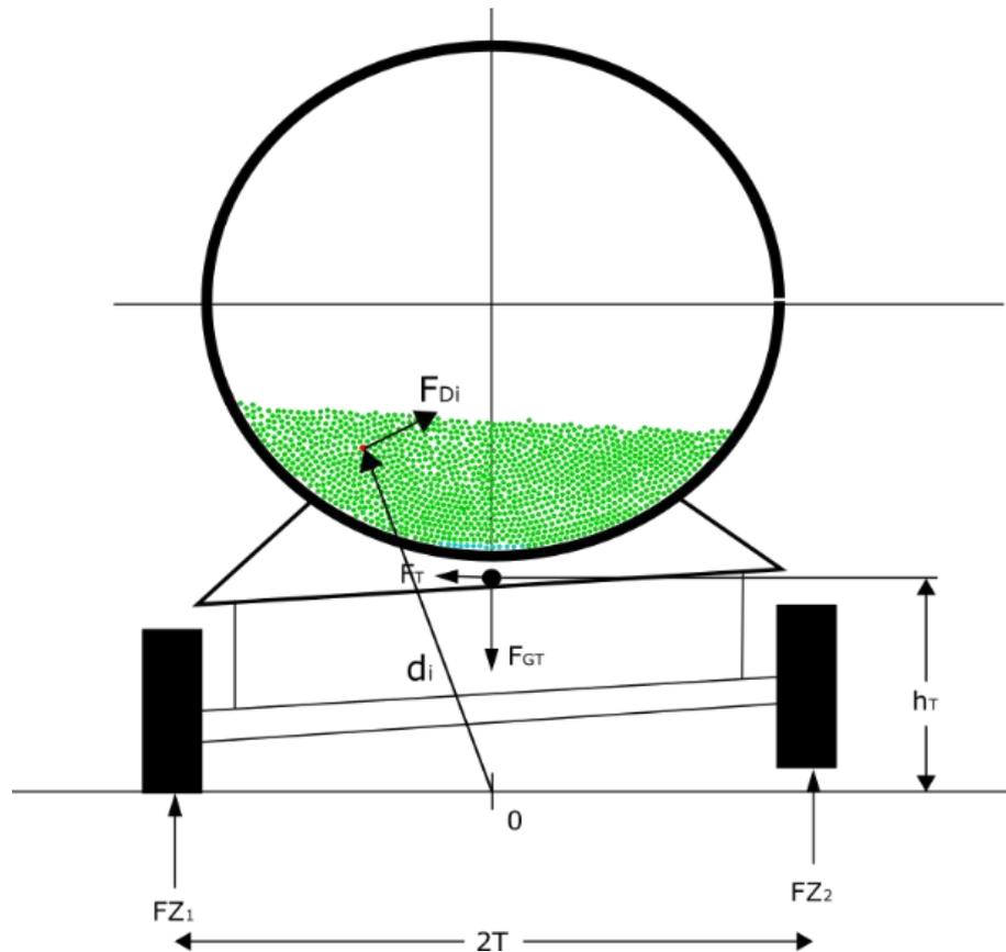
**Figure 3:** Overturning mechanism in the SPH method.
