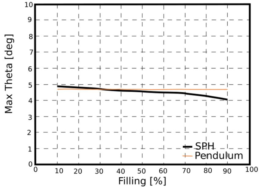
**Figure 6:** Manoeuvre 1: maximum gravity centre inclination as a function of filling height.
