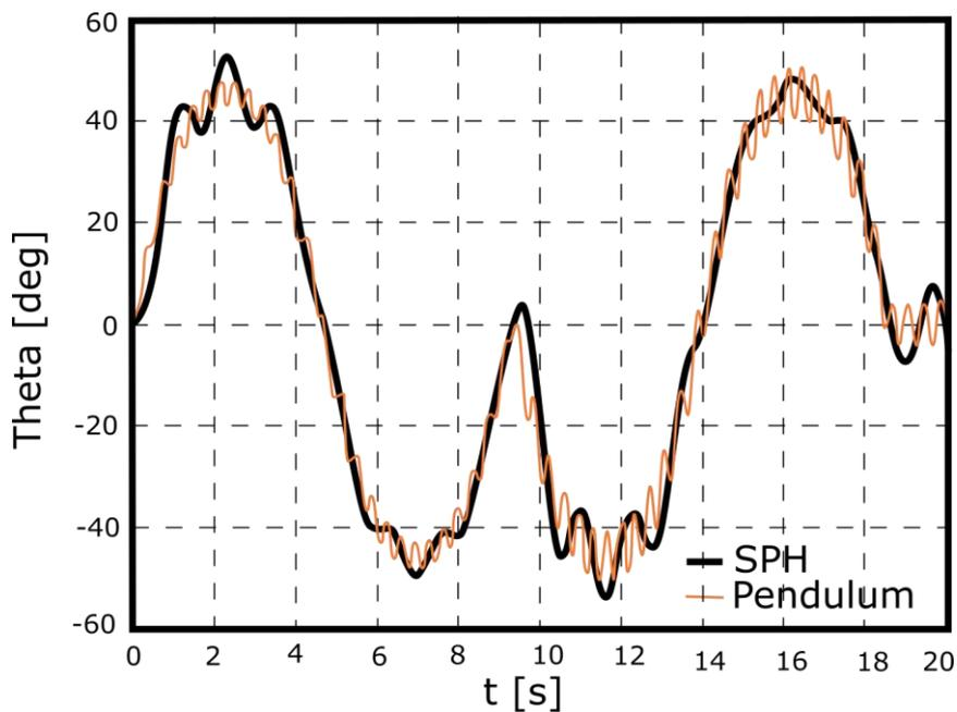
**Figure 8:** Manoeuvre 2: comparison of gravity centre oscillations between the SPH and dynamic pendulum; 80% filling height.
