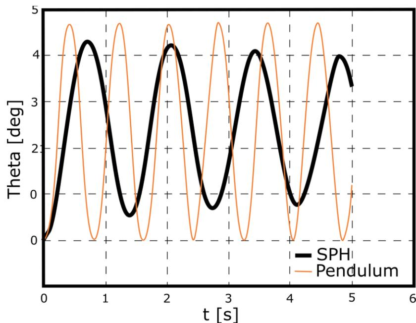
**Figure 5:** Manoeuvre 1: comparison of gravity centre oscillations between the SPH and dynamic pendulum; 80% filling height.
