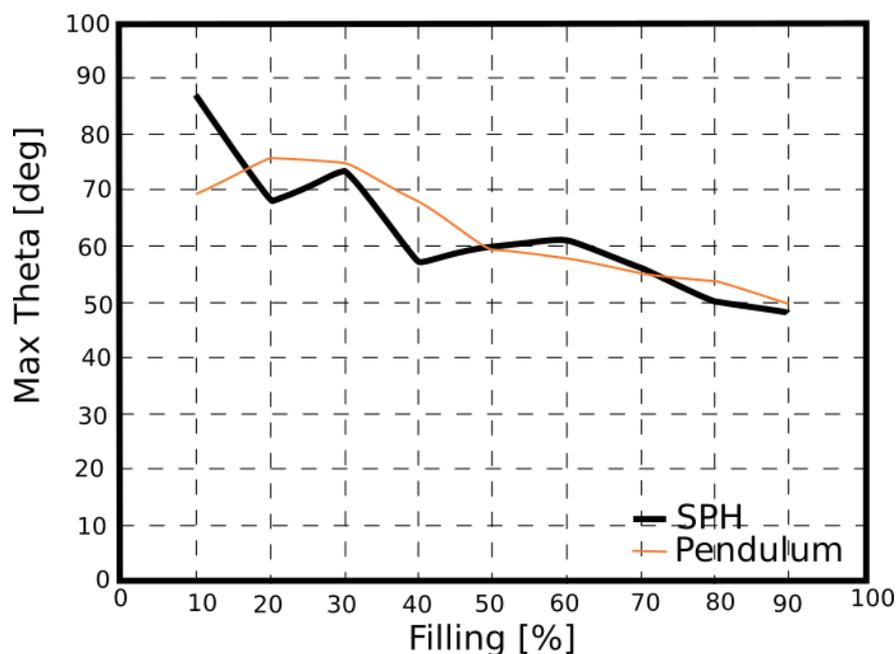
**Figure 10:** Manoeuvre 2: maximum gravity centre inclination as a function of filling height.
