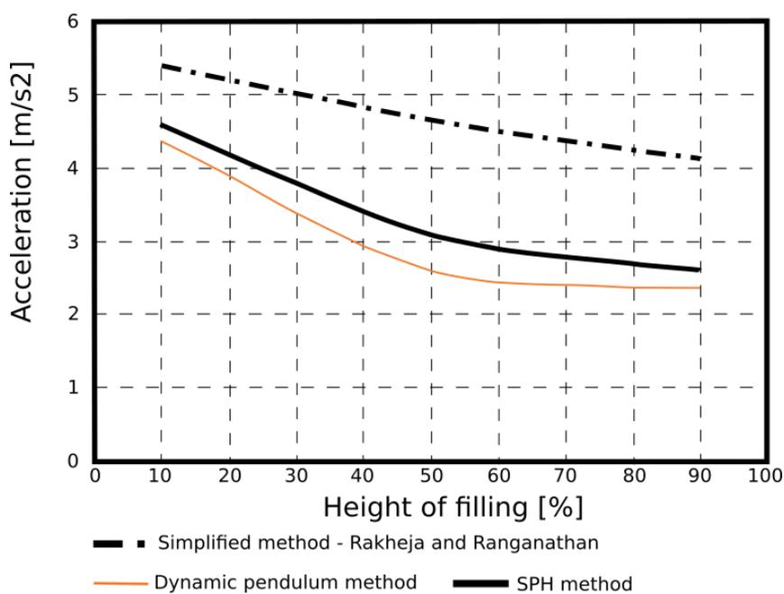
**Figure 11:** Overturning threshold – acceleration vs. filling height; comparison between quasi-static and dynamic pendulum, and the SPH methods.
