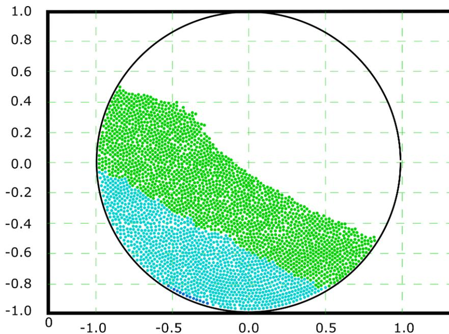
**Figure 9:** Manoeuvre 1 (overturning threshold determination): position of particles in time  $t = 3.8$  s; 50% filling height.
