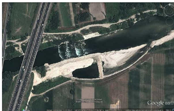
Figure 7: The riverbed ramp downstream of the Šentjakob Highway Bridge after the Sava 2012 Flood. The flood caused a local right bank cut downstream of the ramp; the repair works have already been done (source: Google Earth, July 17, 2013).
